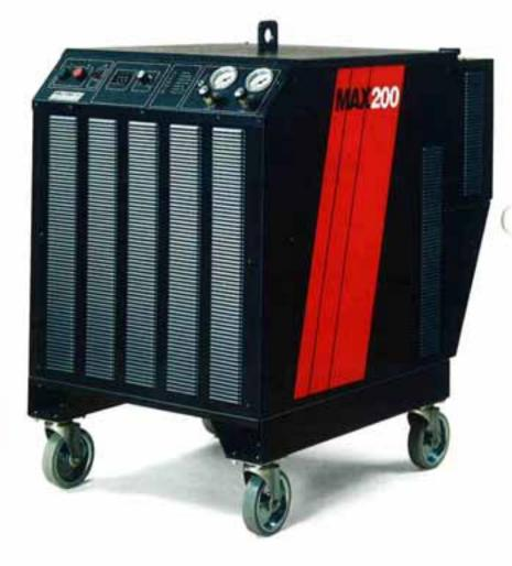
The MAX200's patented shielded torch front-end practically eliminates the possibility of double arcing, greatly enhancing piercing capabilities and extending consumable parts life.
