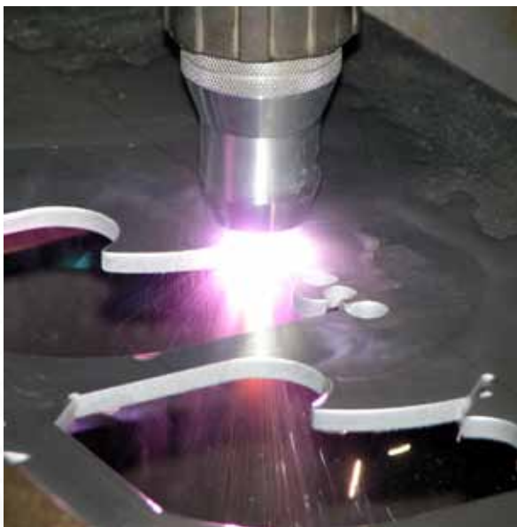
Cutting Aluminum with the Ultra-Cut® 200
